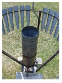
Wind screens are added to slow the wind and reduce problems caused by localized winds that are created by a rain / snow gauge disrupting the small to microscale wind field around the gauge. As shown in the following diagram, wind perturbations can carry precipitation over and beyond the rain gauge (the grey box in the image below). This can lead to smaller precipitation accumulations in the rain/snow gauge than in the area just around it.
